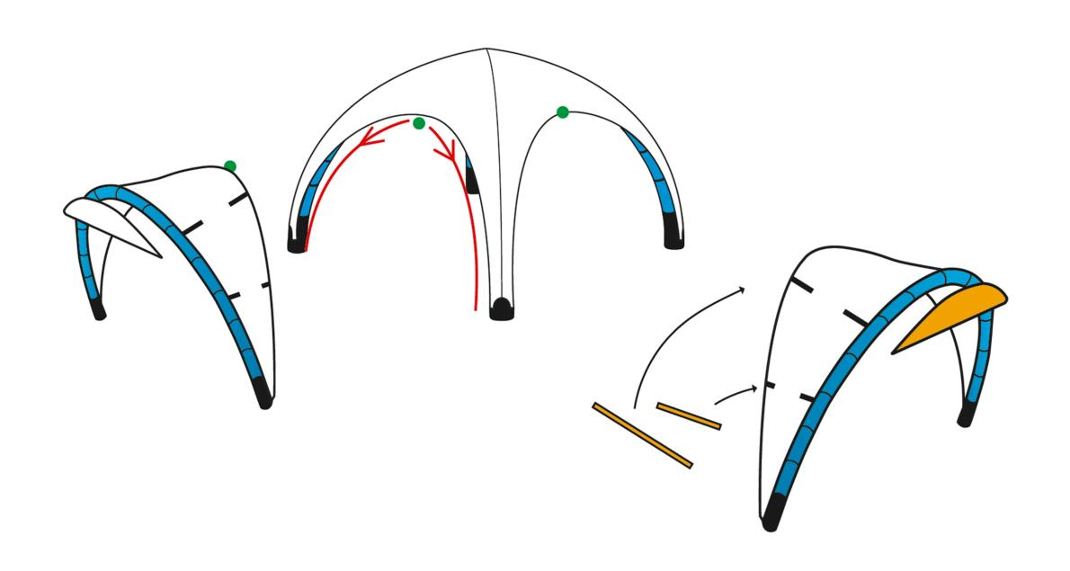
**Tent Connector setup:** Once both tents to be connected are inflated and positioned facing each other, unfold the connector and and zip it beginning from top to bottom connecting it to the tent-arches. Connecting tents highter than 4x4 requires a ladder or another kind of platform to close the zippers.
