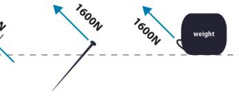
**8.** Pins and pegs should be hammered into the ground under 40° (±5°) angle and - ideally - stick out above the surface no more than 25mm. They need to sit firmly in the ground.
