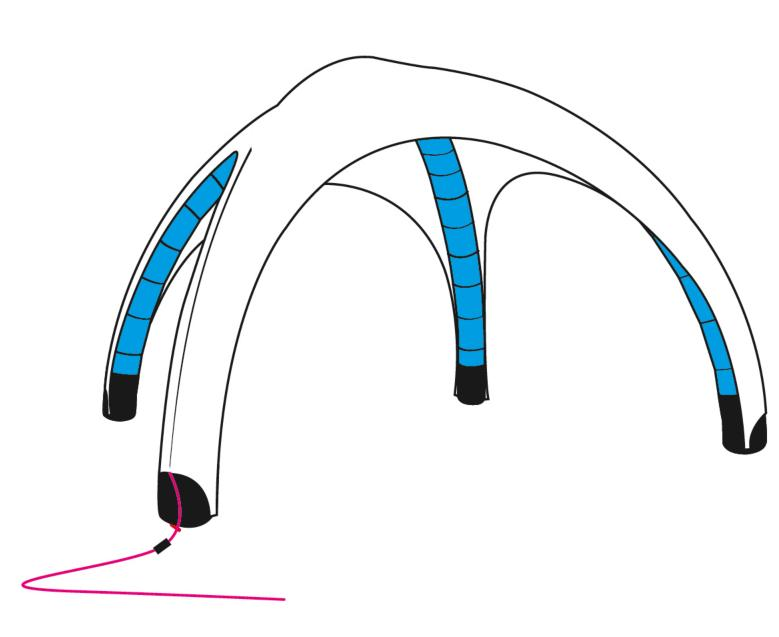
Finally attach the cable at the bottom of the leg to the adapter with the 230V cable (d.).
