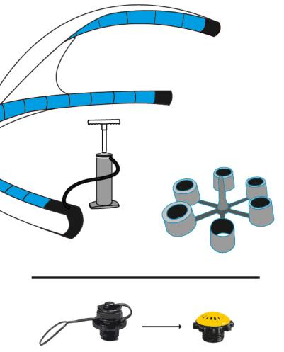
**4.** Fit in the end of the pump's hose into one of the valves and begin the process of inflation (you may need to use the adjustment fitting for the pump to fit the valve opening). The one-pump system will let the air to slowly fill in the remaining legs.
