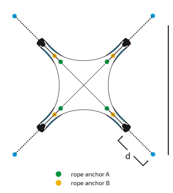
**7.** Even though not necessary in milder winds, we strongly advise you to always use awning anchoring (together with primary anchoring). It provides better wind-resistance and secures the tent against sudden wind gusts.
