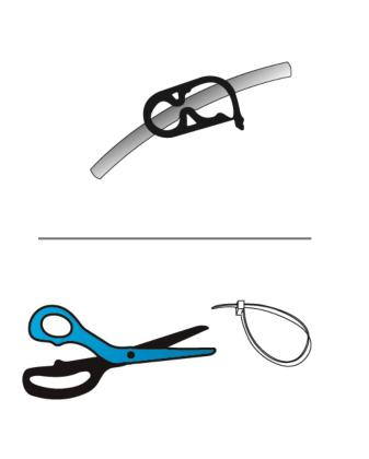
Bladder repair A: Before you proceed with bladder repair make sure that the air leak is not due to a valve problem. Once you are sure it is one of the bladders proceed to identify the one that leaks - use the stopper clamps attached to rubber pipes to block the air flow and check each bladder separately.
