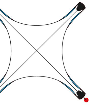
6. As soon as you set the tent's legs in the desired position you should secure the tent to the ground. You may choose one of two primary anchoring systems: ballasts or pins.
