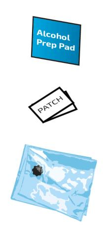
Bladder repair B: Before you begin the repair, make sure you located all the punctures, tears or abrasions. You should use airflow plugs to block the airflow through the one-pump system valves and search for leaks in perfect silence. Alternatively you may submerge part after part of the inflated bladder in water or sprinkle it thoroughly with non-agressive household detergent and search for bubbles of air leaking.
